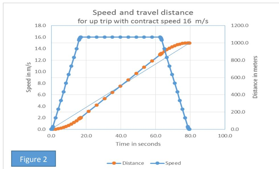
For this trip, the periods for acceleration and deceleration are 17 seconds each plus 46 seconds at 16 m/s. The total car flight time is 80 seconds. The straight line between level zero and 1000 m shows the internal air pressure of the airtight car, which declines as if the car is travelling at 12.5 m/s.
